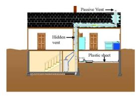
A contractor will route the vent pipe in such a manner that if, after the home is tested and the levels are not acceptable, a fan can easily be installed in the vent pipe within the attic to make the system more effective.
